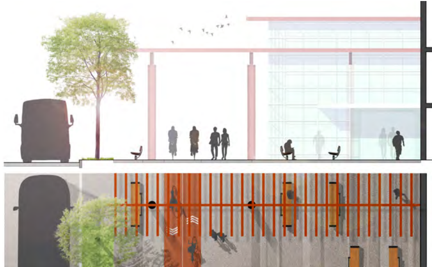
Separated bicycle lane at hub: Bicycle lane is separated from vehicular traffic
